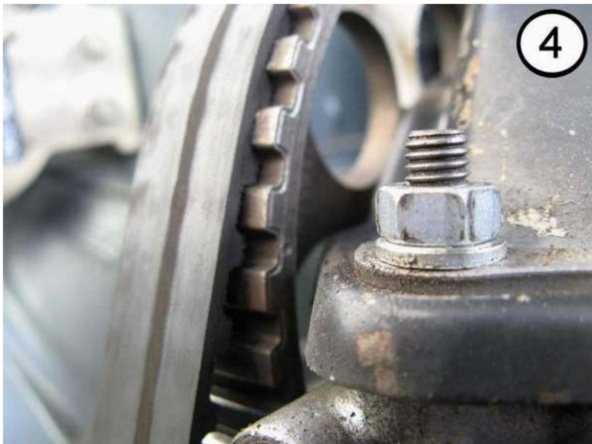
Cam timing mark, Mk1 and early Mk2 with steel belt covers (note the dot is level with top of valve cover installed)
