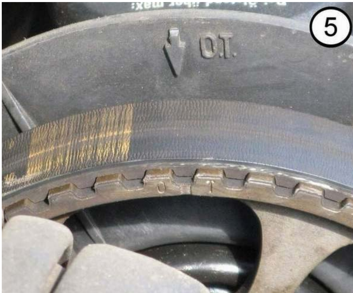
Cam timing mark Mk2 and Mk3 (clip on timing belt covers)
